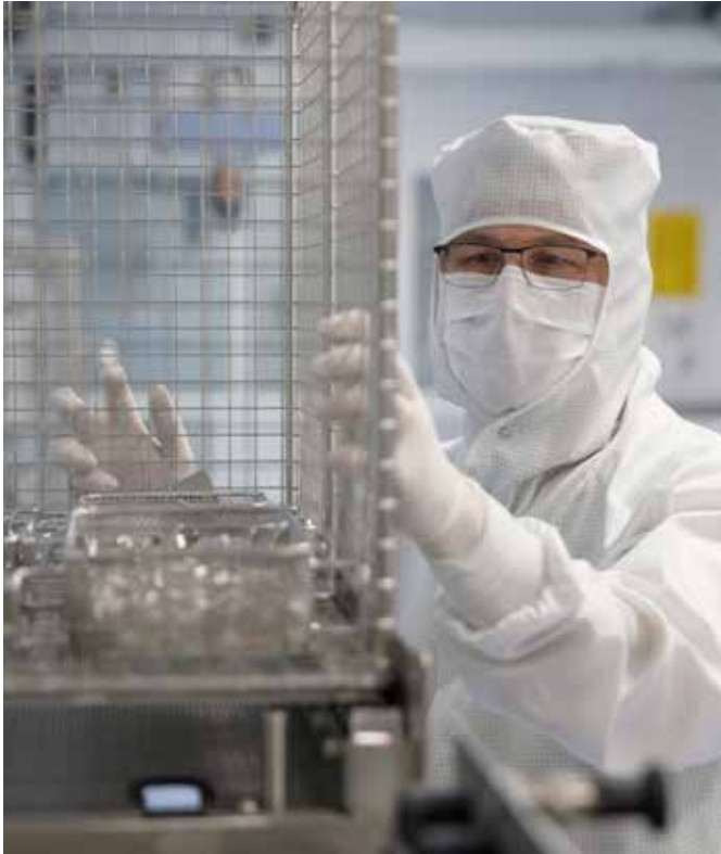
Cleaned components are transferred to the ISO 5 cleanroom for assembly.
