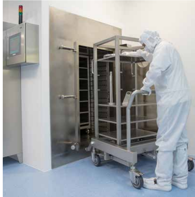
Dry cleaning by baking in the vacuum oven ensures highly clean surfaces.
