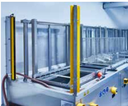
Wet cleaning in the class 6 cleanroom: the components are provided on entry with a badge for identification and documentation.
