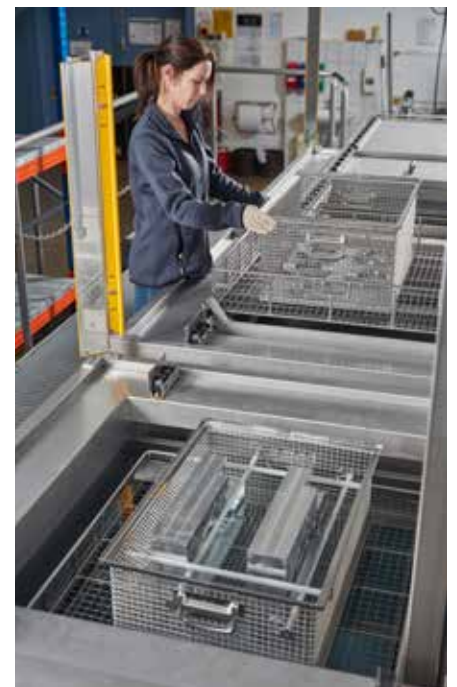
Ultrasonic cleaning bath at ALMA Plant I
