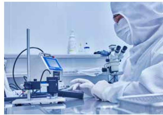
Visual inspections for particle contamination can be performed with white or UV light as well as with a CleanoSpector or light microscope.
