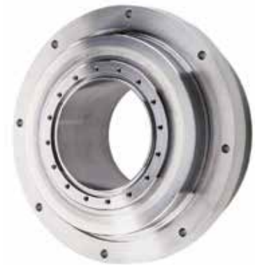
ALMA flange, hollow shaft, very flat design with a large internal diameter, integrated roller bearings for extremely high loads
