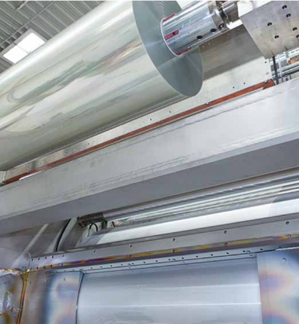
With FlexBlue sputtering systems from SCHMID, various metal and non-metal films can be applied onto flexible substrates from roll to roll in a vacuum.
