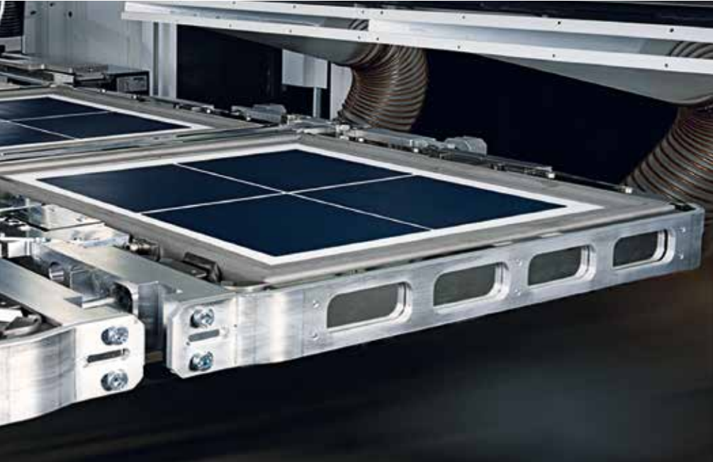
The VCS 1200 PECVD (plasma-enhanced chemical vapour deposition) system coats the front and rear of silicon wafers. (Photo: MANZ AG, Corporate Communications)
