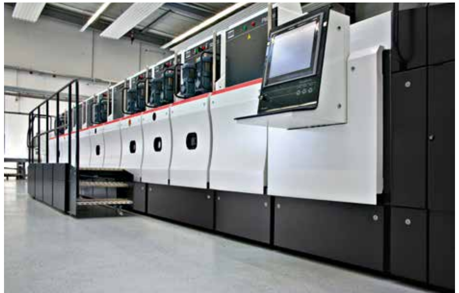
PIA | nova® – modular platform for the coating of glass for thin-film photovoltaics. (Photo: VON ARDENNE Corporate Archive)
